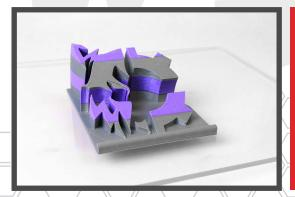
AS PARTS COOL THEY WILL BEGIN TO "POP" OFF OF THE GLASS. DO NOT BE ALARMED, AS THIS IS JUST THE SOUND OF THE PARTS RELEASING THEMSELVES FROM THE WOLFBITE SOLUTION. COLD WATER WILL SPEED UP THE PROCESS, BUT MAKE SURE TO LET THEM COOL IN AMBIENT AIR FOR A FEW MINUTES FIRST.
