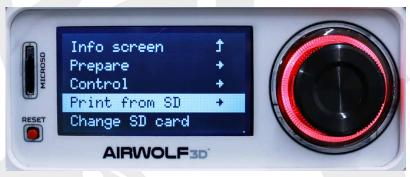
Using the scroll wheel, choose the file named **NOZZLE 1 FINAL PRINT**. AXIOM Dual will then preheat to the proper printing temperatures and begin the auto-leveling process. Once complete, the print will start and the model will begin printing.
