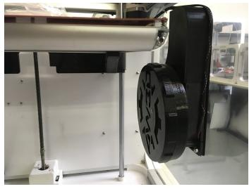
6. Screw on the filter and filter cover.
