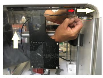
2. Bring the fan wire up, through the zip tie and through the back panel of the machine.
