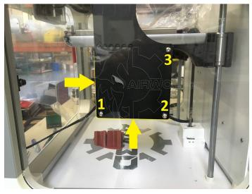
Hold the fan assembly on the inside and position the bottom and left edges square on the logo.
