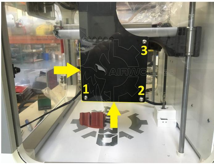
1. Hold the fan assembly on the inside and position the bottom and left edges square on the logo. Mark spots with a sharpie, drill out with a 5/32 in bit and attach with the three screws.
