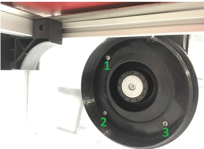
5. Unscrew the two HEPA filter pieces and attach the inner one to the inside of the machine with the three screws.
