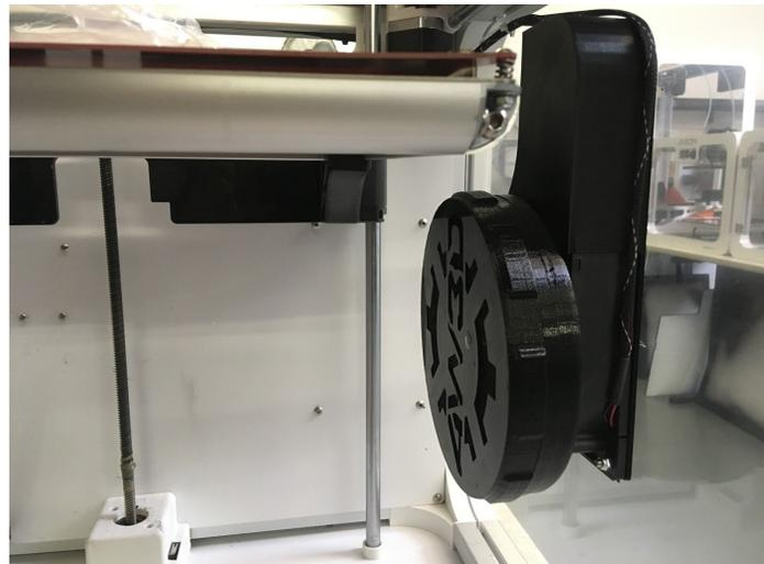
6. Screw on the filter and filter cover.
