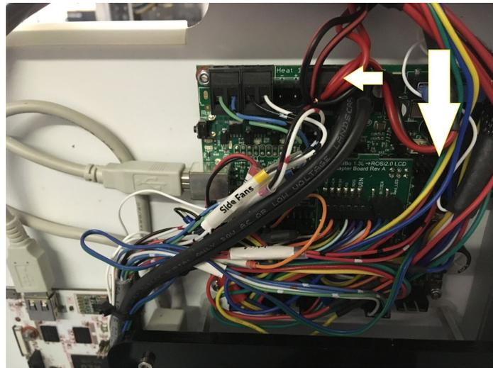
4. Unplug the power wires from port "Fan 1" and remove the connector from the wires. Twist the fan wires to the other wires and reattach the connector
