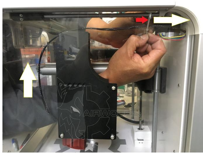
2. Bring the fan wire up, through the zip tie and through the back panel of the machine.
