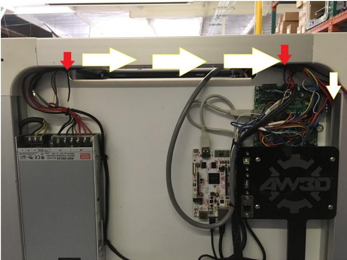
3. Run the fan power following the other power wires through the top edge. Secure them with two zip ties.
